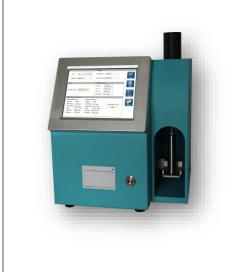
Using industrial camera, machine vision technology, automatically Automatic identify smoke point and flame height. High precision and good repeatability
